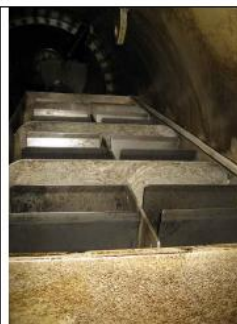
Inspection area #1: The non-ret valves in the scavenging air recei should be photographed. Comment:
